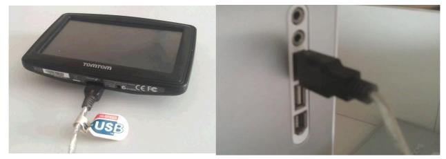
Connect the GPS using the supplied USB cable.
